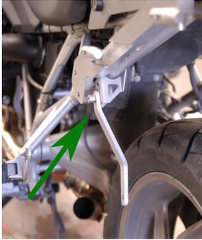
First, attach the short end of the Exhaust Hanger to the bike. The Exhaust Hanger should bend in towards the bike. Attach it in place with the M8 x 20 allen head cap screw and the M8 split washer. Keep all connections loose at this point. All connections will be tightened at the end of the process.
