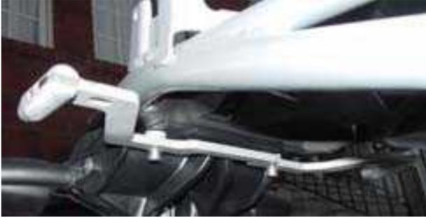
Attach the “W” bracket to the frame of the bike. The tapered end of the bullet connectors on the “W” bracket must be facing towards the back of the bike.
