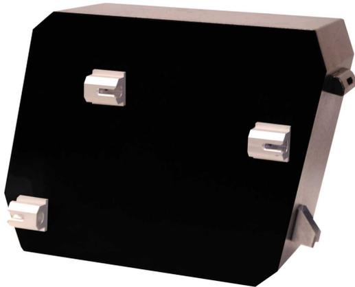
Using the M5 x 16 button head screws, with M-5 split washers, attach the backing plate to the mounting block. With the backing plate inside the case and the case mounting blocks outside the case, assemble loosely, using a 3 mm Allen key. These screws will all need to be tightened after final fit up. See photo below.
