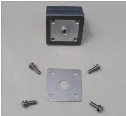
After each block is mounted, insert the black securing knob through the locking tab and into the center hole of the case mounting blocks, from inside the case. Use anti seize on the thread of the thumbscrews to prevent corrosion. See photo below.
