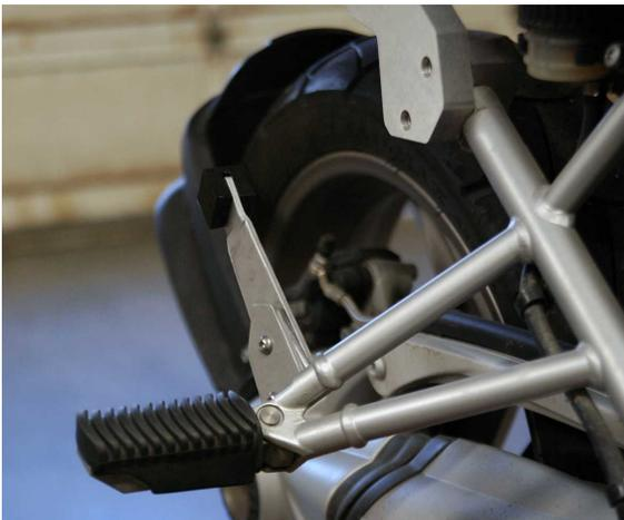
Using a 4 mm Allen wrench, remove the bolts holding the two pieces of the right foot peg extension. Position the larger piece on the inside part of the foot peg bracket. Note: the flat head screw securing the black spacer will face inwards towards the wheel. Position the smaller plate on the outside of the foot peg bracket, which is the side facing you. Insert and thread both bolts using only hand pressure, to ensure you do not cross thread them.
