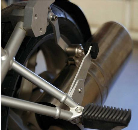
Follow the same installation as the right side mounting plates. Note: the flat head screw securing the black spacer will face inwards towards the wheel.
