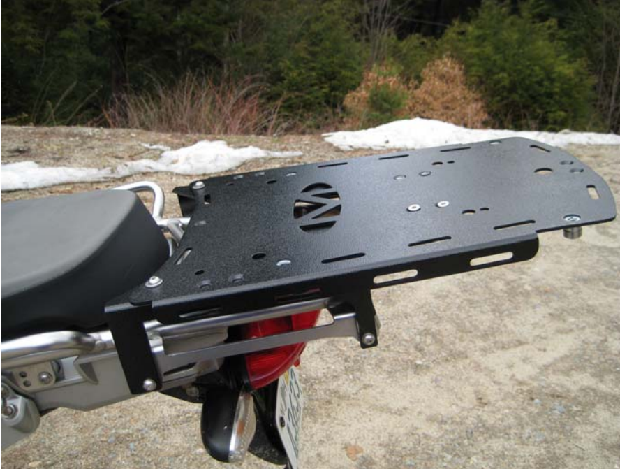
Micatech Pack Rack, Mounted in Rear Position on BMW R1200GS Adventure Rack
