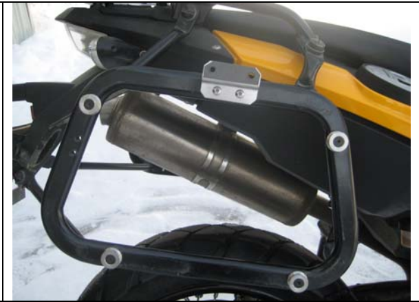
Photo 5: Hold-down bracket mounted for V2 higher position
