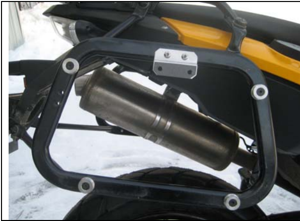
Photo 4: Hold-down bracket mounted for V2 lower position
