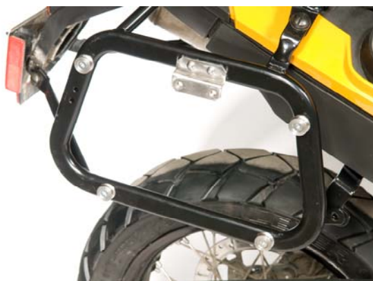
Photo 1: Rack and hold-down screw mounted in lower position
