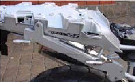
Rest the rear end of the right side frame on the protruding end of the “W” bracket, next to the bullet connector. Do not insert the M 8 x 25 fastener into the bottom of the right side frame just yet. Insert the M6 x 45 screw into the appropriate hole near the back of the frame. Be sure to place the 15 mm spacer in the space between the hole in the frame and the threaded hole in the motorcycle frame. Partially thread this bolt into the corresponding hole in the bike frame.
