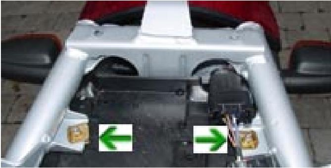
Now, go back to the area above the wheel well, and under the stock bag mount platform that you have just removed. Using a flat head screwdriver, push and slide the two corresponding securing tabs towards the opposite side, and remove them. Re-attach the two bolts you have just removed to their securing tabs and store them with the stock bag mounts. You will not be using them again.
