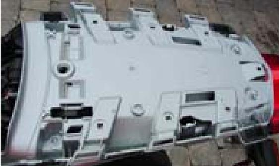
Re-attach this platform using its four Torx 30 bolts, and Torx 25 to secure the seat lock mechanism.
