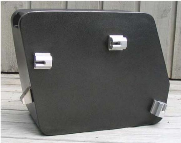
Using the M5 x 16 button head screws, with M-5 split washers, attach the backing plate to the mounting block. With the backing plate inside the case and the case mounting blocks outside the case, assemble loosely, using a 3 mm Allen key. These screws will all need to be tightened after final fit up. See photo below.
