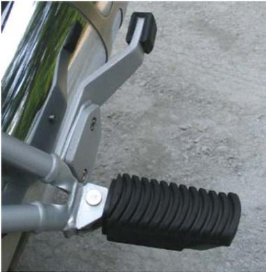
Follow the same installation as the right side mounting plates. Note: the flat head screw securing the black spacer will face inwards towards the wheel.
