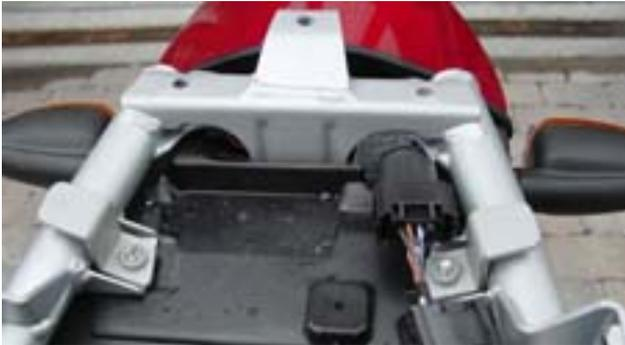
Place the two small Z shaped brackets over top of the holes, on the frame side of the bike. The two horizontal tabs in the Z bracket must be just over the top of the round frame tubes.
