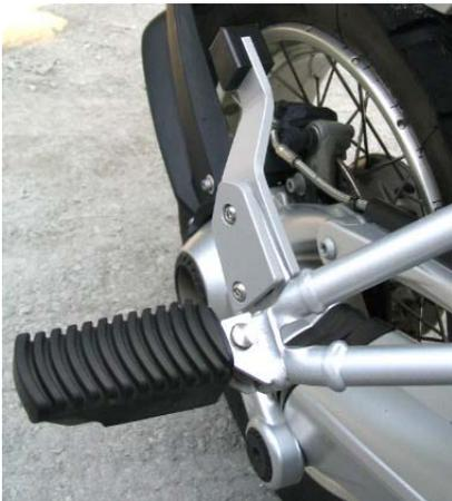
Using a 4 mm Allen wrench, remove the bolts holding the two pieces of the right foot peg extension. Position the larger piece on the inside part of the foot peg bracket. Note: the flat head screw securing the black spacer will face inwards towards the wheel. Position the smaller plate on the outside of the foot peg bracket, which is the side facing you. Insert and thread both bolts using only hand pressure, to ensure you do not cross thread them.
