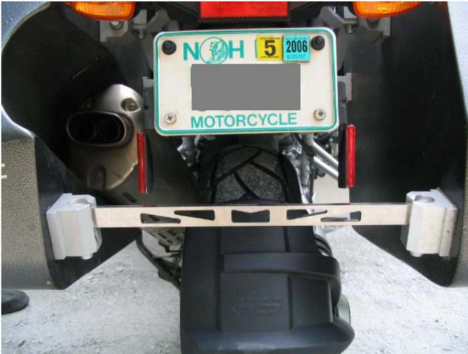
Once you are satisfied with the fit of the cases on the mounting bullets and the foot peg extensions, install the lower rear support bracket. You need to insert both bullet connectors on this support bracket simultaneously into the lower mounting blocks. This is easily done by gently pushing the cases outwards, as you slide the bullet connectors into the mounting blocks. Once you're satisfied with the final fit, remove the rear cross bar and slide the cases on and off to ensure a good fit.
