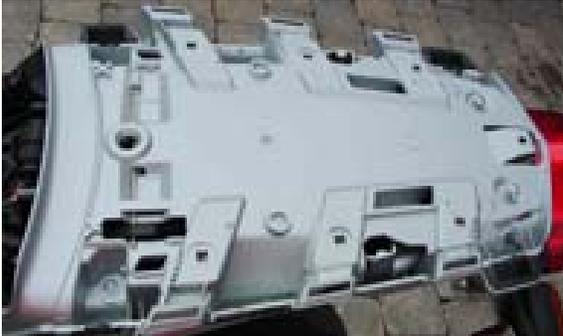
There are five bolts that need to be removed here. Using a Torx 30 wrench or socket, remove four screws and related washers. For the last fastener, you need a Torx 25 to remove the seat lock holder. Carefully store all bolts and remove the stock bag mount platform.
